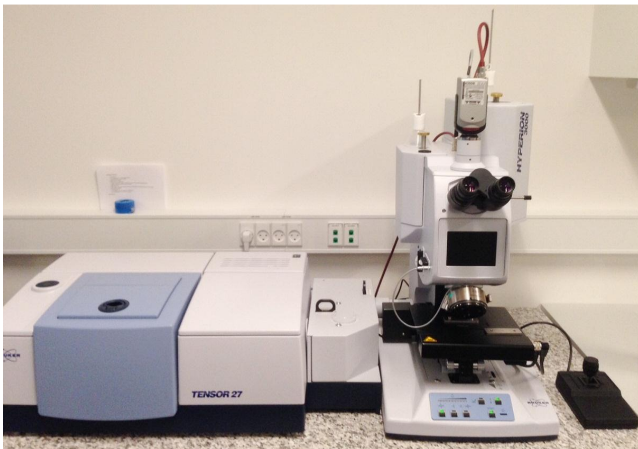
The FTIR Hyperion 3000-TENSOR 27 with a FPA detector ready for analysis at the CATS labs, SMK.
