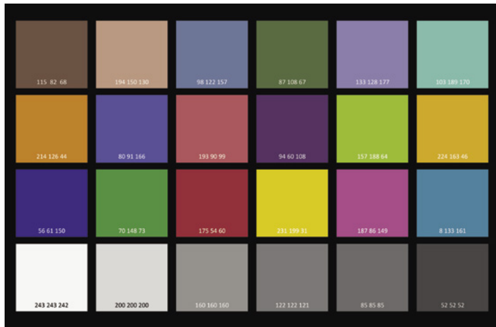
Fig. 4 X-Rite Macbeth ColorChecker Chart. Middle values chosen for DttG system, based on manufacturers' sRGB D65 values, are white: #f3f3f2, black: #343434, red: #af363c, green: #469449, yellow: #e7c71f, blue: #383d96, brown: #735244, purple: #5e3c6c, pink: #c15a63, orange: #d67e2c, and grey: #c8c8c8, with the 'light' and 'dark' modifiers varying by 20% in brightness.
